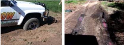
Next Ade decides to place one front wheel of his Patrol over Ruedi's sand anchor to increase the resistance of the anchor and at the same time pull with the Patrol's winch. Slowly the wheel sinks into the sand as the OKA starts pulling the Patrol, but all of a sudden the OKA starts moving out of its bog and shortly after is back on the track.
