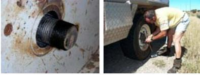
All the threads are damaged but since the nuts are harder than the studs, Ruedi can rethread them with grease and lots of muscle power.
