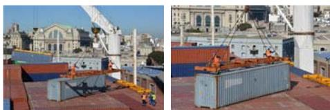
Here too the container carrying mechanism is lowered to "load" two people that have to push the mechanism around in such a way that it can clicks itself onto the container at the correct position.
